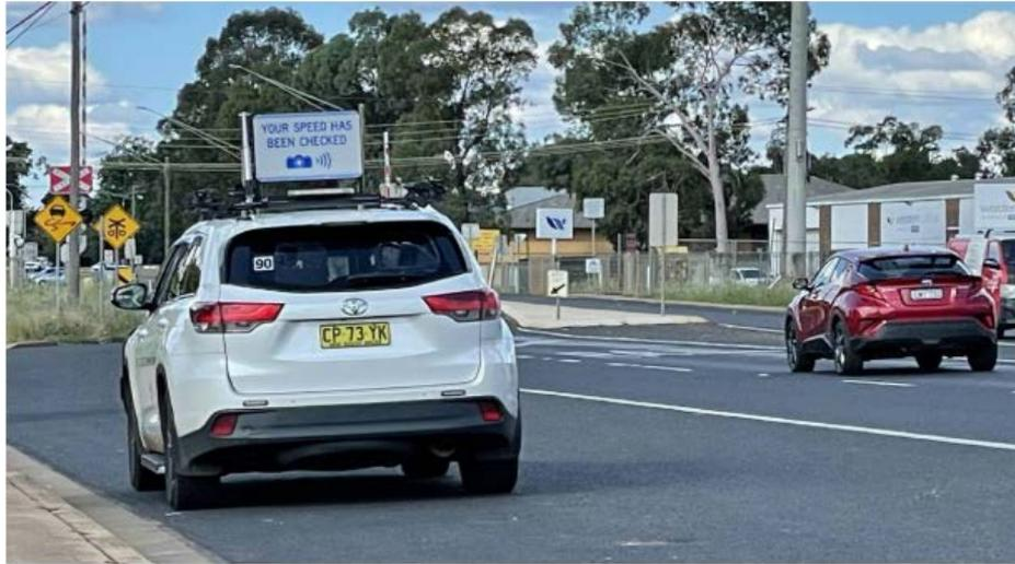
Figure 1: Retractable warning sign on detection vehicle on Cobbora Road in Dubbo<sup>38</sup>
